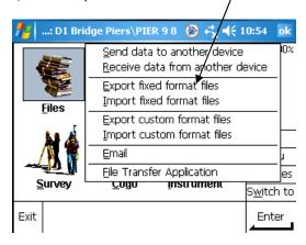
3) From dropdown list under File Format select SDR33 DC. File name will have job name with and SDR extension then tap Accept. The file will be put in to an Export folder in the Job folder. If you don't have a job folder set up it will be in an Export folder under the Trimble Data.
